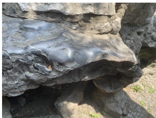
Figure 5. Oxide layer on surface of rockery
