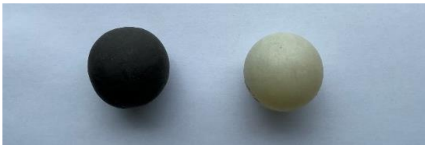
Fig. 3 A 9 grams black ball (left) and a 3 grams Ping Pong ball (right) with the same volume (Photo credit: Original).
