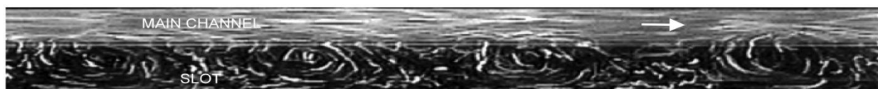
Figure 5. Visualization of Eddies moving from left to right in the longitudinal slot [4]
