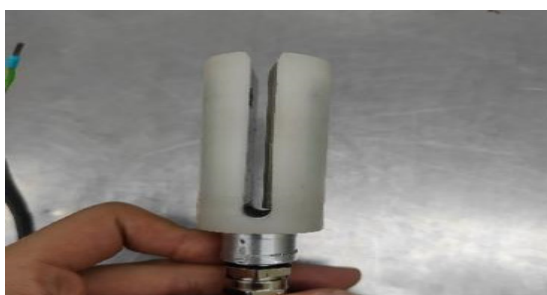
Fig 5. Photoelectric sensors of the tipping paper joint detection system
