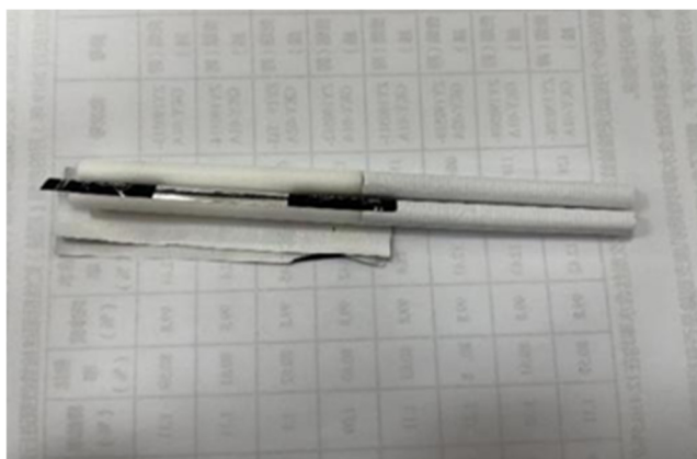
Fig 6. Diagram of a cigarette with a watered-down paper joint
