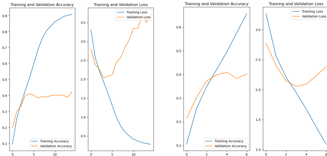
Fig. 4 (left) Training process with overfitting Fig. 5 (right) Training process with early stopping implemented
