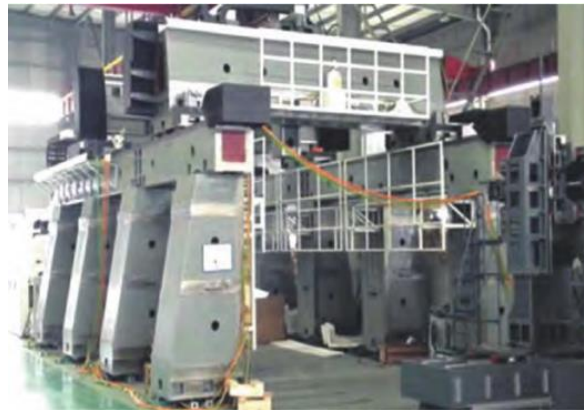
Figure 2. Multi-channel deposition of "bridge-type" additive manufacturing equipment [5]
