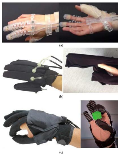
Fig. 1 shows close-up views of various exoskeleton gloves: (a) the Exo-Glove Poly; (b) a flexible rehabilitation glove, the work of the National University of Singapore; and (c) the Compliant Hand, a novel pneumatic actuator-based design by Harvard University [1].
