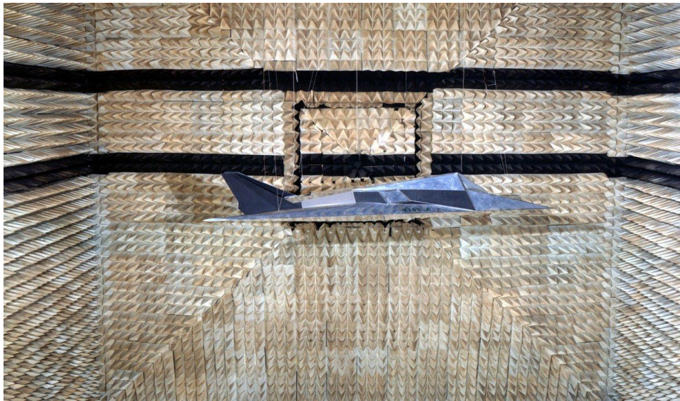
Fig. 1 The Lockheed Have Blue prototype undergoing RCS testing in an anechoic chamber
