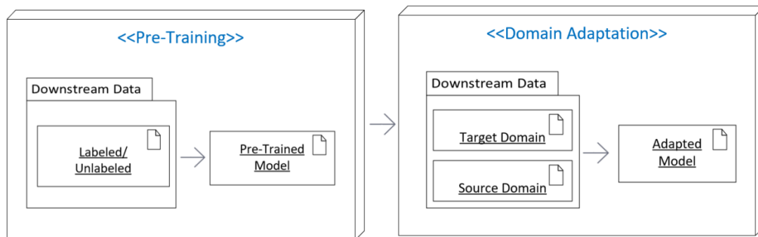
Figure 1. Deep learning applications typically undergo two distinct phases: the first phase involves utilizing a Pre-Trained Model, which serves as the backbone network to learn from large-scale datasets and acquire transferable general knowledge. The second phase is known as Fine-Tuning, where model parameters are adjusted to align the acquired source knowledge with the target network for specific downstream tasks in the target domain. This stage generally requires a certain amount of labeled data relevant to the target field. In cases where there is an insufficient quantity of labeled data for the downstream task, it is possible to leverage source domain labeled data that comes from different distributions but pertains to similar tasks; this approach can enhance model performance on the target task through transfer learning techniques
