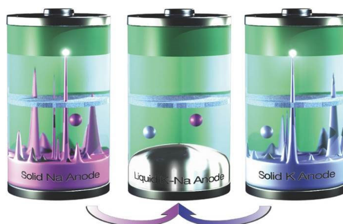
Figure 1-1 Schematic diagram of potassium-sodium liquid alloy anode concept battery [6]
