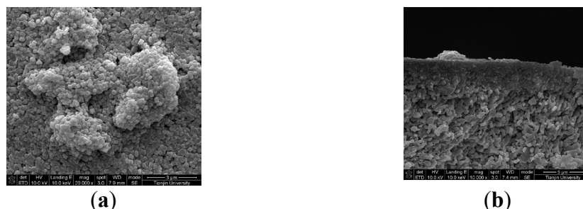
Figure 2. SEM images of the membrane (a) top view and (b) cross section (seeds layer upwards)
