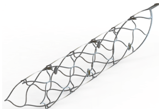
Figure 2. Schematic of a stent-electrode [11].
