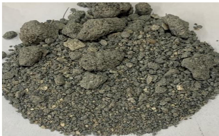
Figure 12. Plugging in well H.
