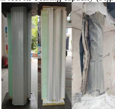
(a) Side in the corridor(before test) (b) Side in the room(before test) (c) Column after test
