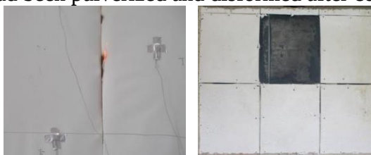
(a) Continuous flame on the back at 100min (b) Fire side of specimen after test
