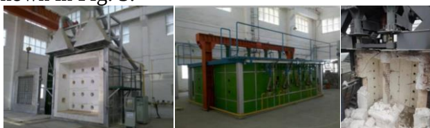
(a) Vertical fire test furnace (b) Horizontal fire test furnace (c) Column fire test furnace
