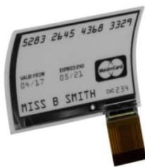
Figure 8. Flexible e-book display based on OTFT device by plastic logic
