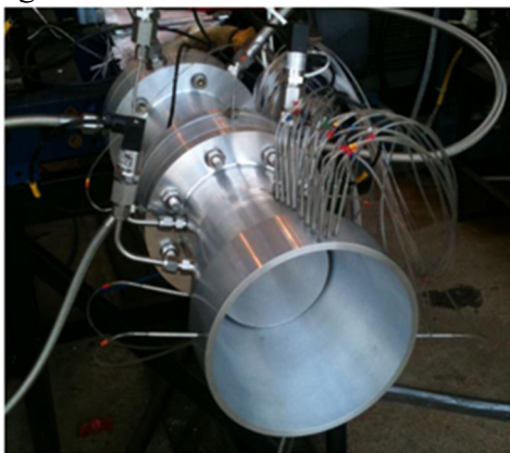
Fig. 2 Strident cold flow rocket engine with dual-throat nozzle [4].
