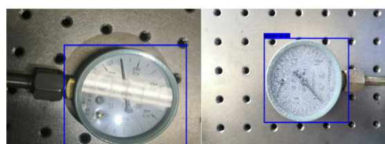
Figure 8. Detection effect of uneven illumination and fog instrument
