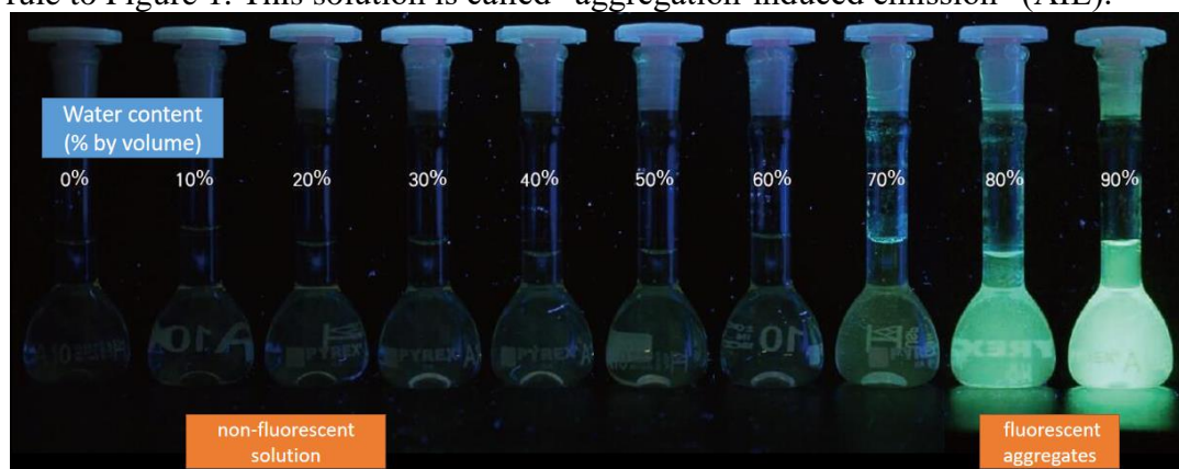
Figure 6. A fluorescent photograph of HPS (concentration: 0.02mol/L) taken under ultraviolet light in a mixed acetonitrile/water solvent with different water volume ratios [12].
