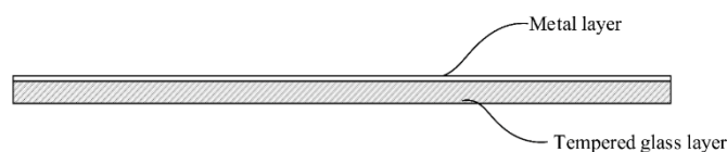
Fig. 2 Structural diagram of tempered glass layer and metal layer before freezing treatment.
