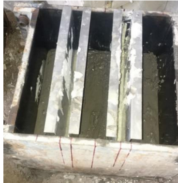
(a) Placing the partition plate
