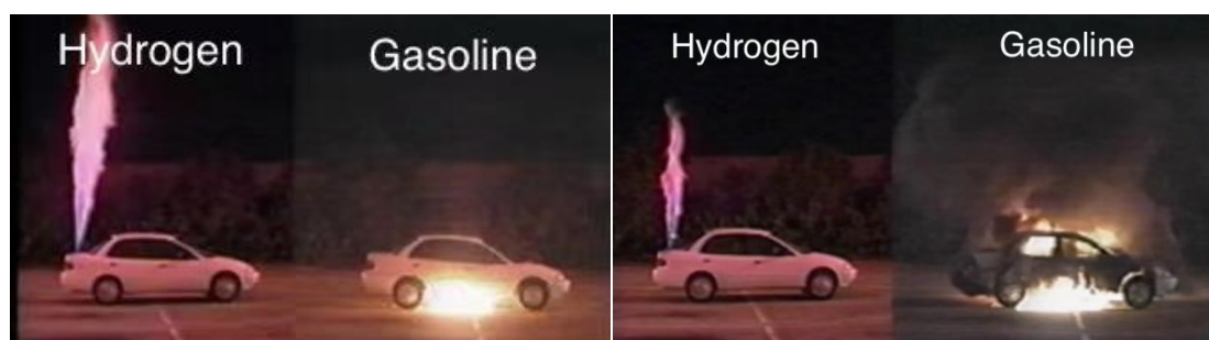
Figure 7. Combustion comparison test of hydrogen fuel cell vehicle and gasoline vehicle [23]. (left: 3s; right: 1min)
