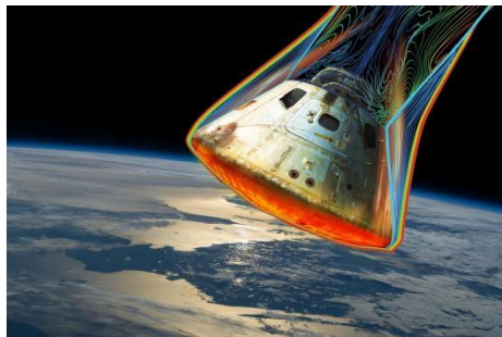
Fig. 3 Distribution Diagram of Aerodynamic Shadow Zone of Return Cabin in Reentry Phase [3]
