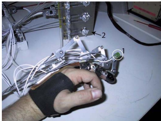
Fig. 3 Prototype of the exoskeleton. Hall sensor and Actuator unit [10].
