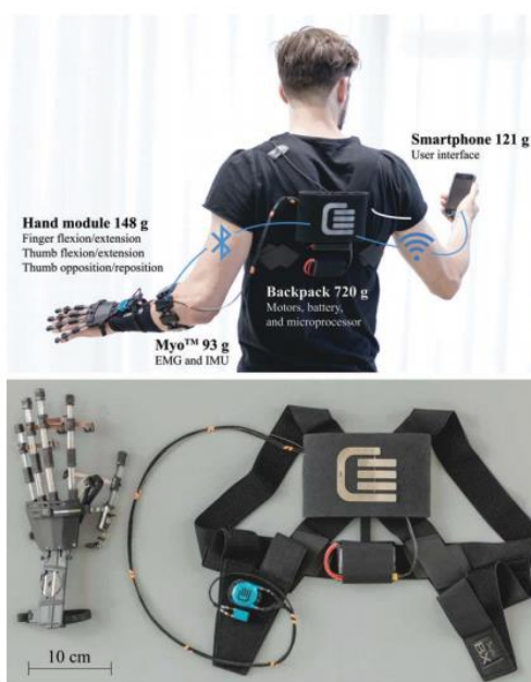
Fig. 12 RELab tenoexo consists of hand exoskeleton and backpack control system [18].
