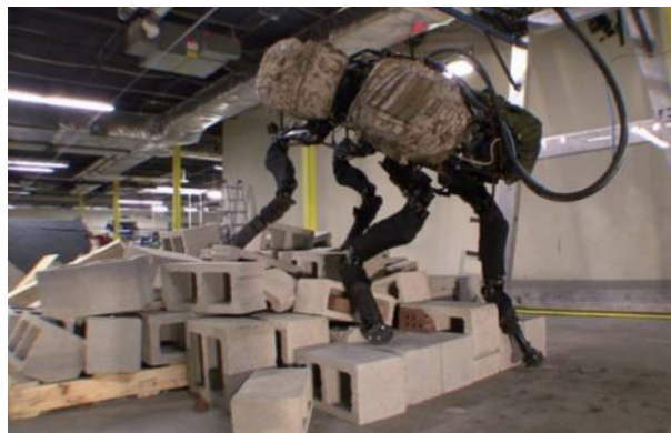
Fig. 3 BigDog climb a rubble pile [4]
