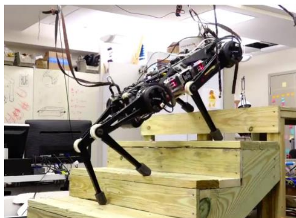
Fig. 4 Quadruped robot climbs stairs [5]
