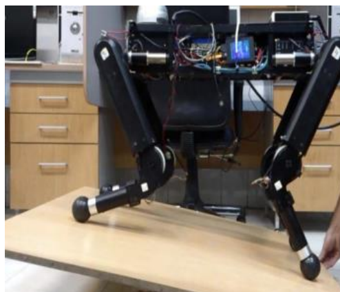
Fig. 6 Attitude Balance of a Quadruped Robot on a Slope [10]
