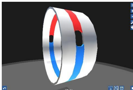
Fig. 9 Bin portholes divided into upper and lower parts
