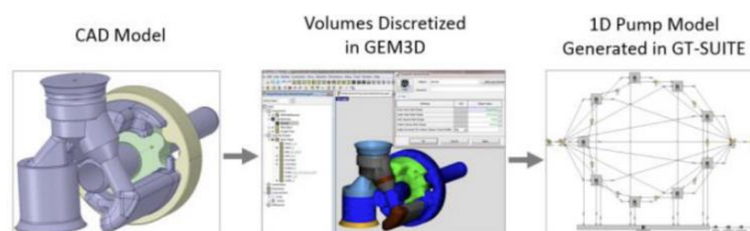
Figure 14. One-dimensional flow models are created by loading CAD models into the GEM3D preprocessor
