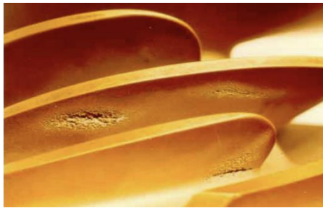
Figure 23. Cavitation damage on a pump blade for mixed flow
