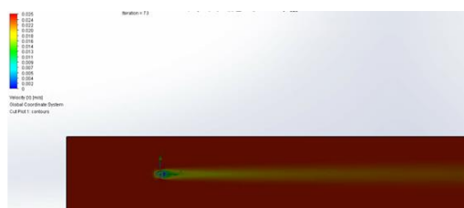
Figure 12. Flow Pattern for Reynolds Number = 100
