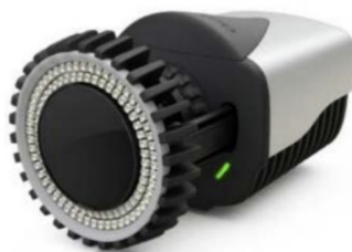
Fig 2. Qualisys OQUS 6+ series passive optical motion capture cameras.
