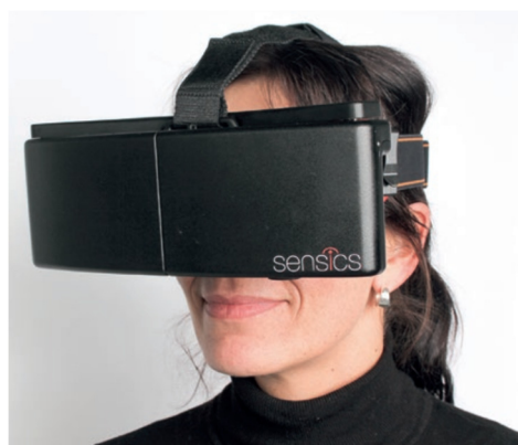
Fig 9. VR headset with integrated Dikablis eye tracking camera
