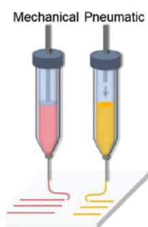
Figure 2. Schematic of extrusion-based bioprinting
