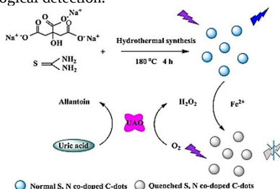
Figure 2 The proposed uric acid-sensing principle [10].
