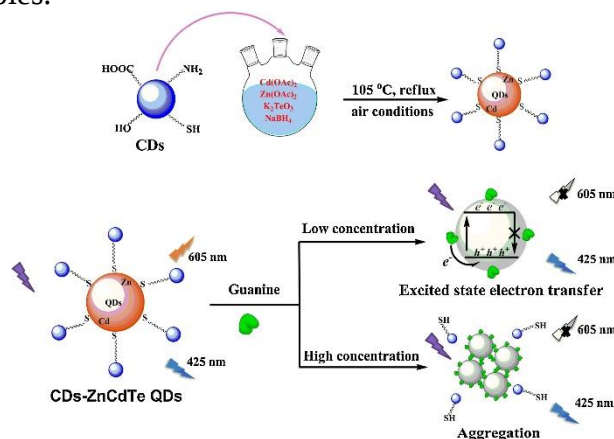
Figure 3 The proposed mechanism of fluorescence sensing for the detection of guanine [11].
