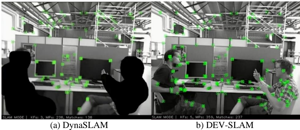
(a) DynaSLAM (b) DEV-SLAM Figure 2. Results of masks and feature points in the walking scenario.
