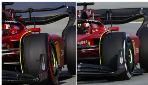
Figure12. DRS system on and off [8].
