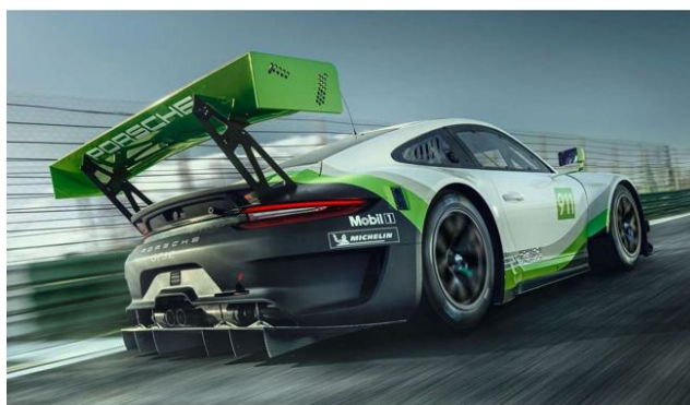
Figure 11. The huge rear wing in the racing car [10].
