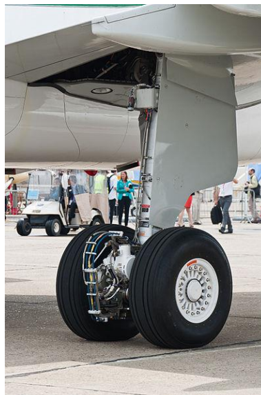
Figure 8. The demonstration of electric taxiing [9]
