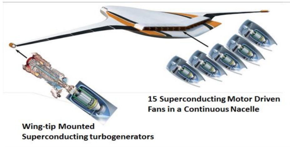
Figure 9. A hybrid aircraft's distributed turbo-electric propulsion system
