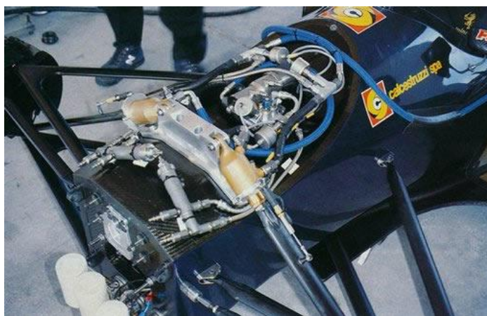
Fig 9. The Minardi FRIC system (Active Suspension) introduced on Minardi M193 in 1993 [15].
