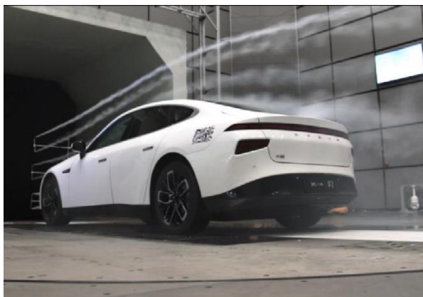
Figure 4. Automotive wind tunnel test.
