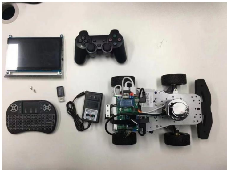
Figure 9. Controllable physical four-wheeled trolley
