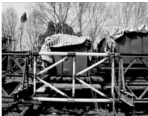
Fig. 3 Static and live load loading site of composite truss piece [7]
