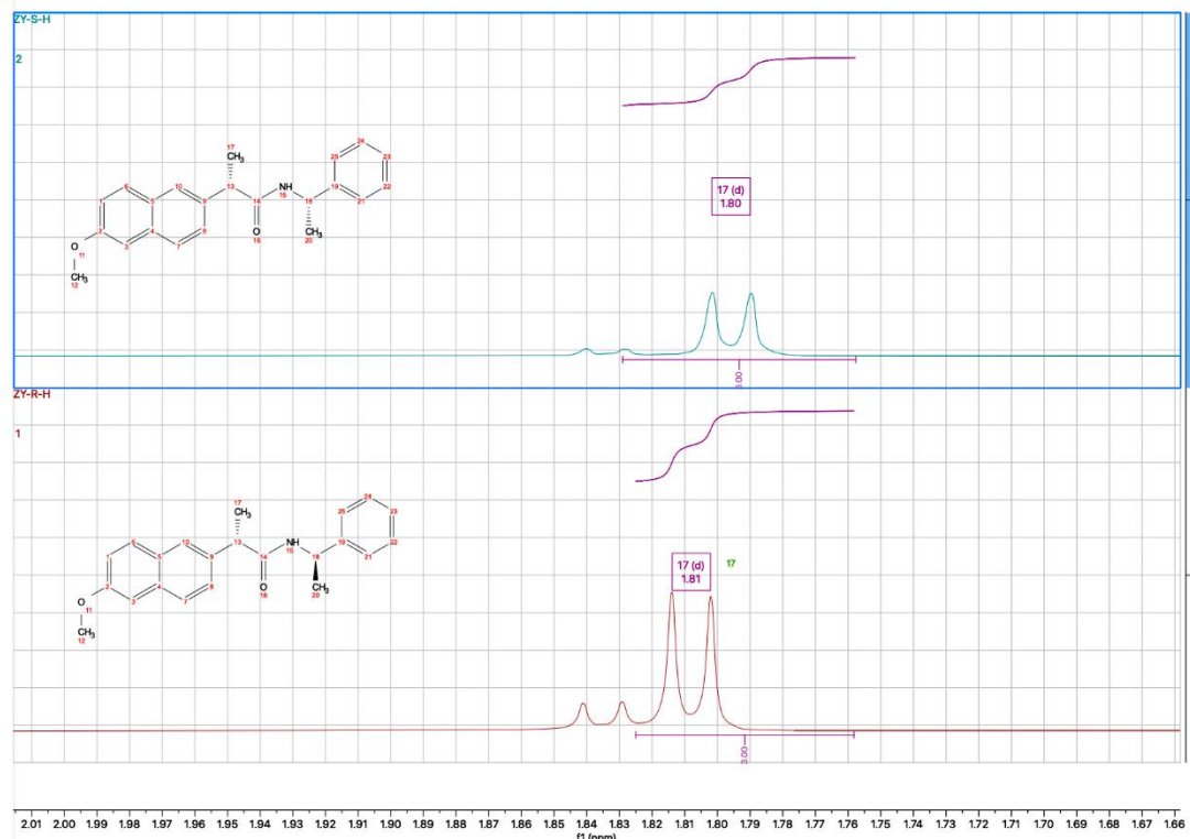
Fig. 6 Comparison of chemical shifts of C(17')H 1 H NMR spectra of compounds 3R and 3S
