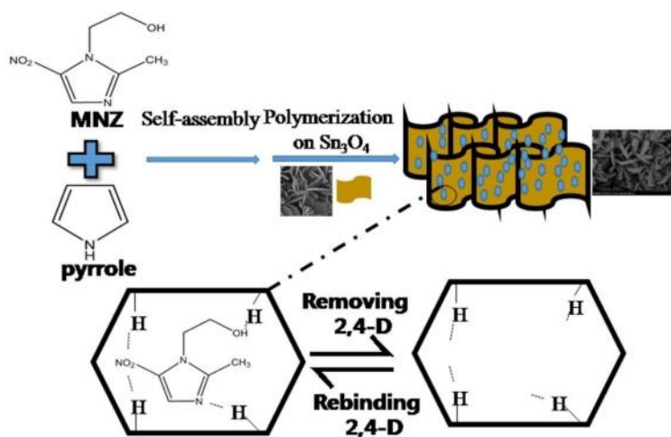
Fig. 3 Preparation principle of MNZ imprinted 2D \text{Sn}_3\text{O}_4 nanosheets [12].
