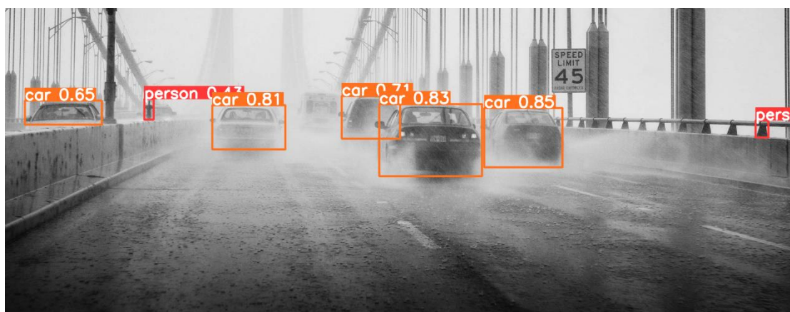
Fig. 4 The detected result of YOLOv5 with the original image-2 (source from [11])
