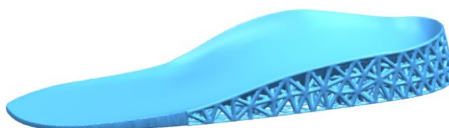
Fig. 3 MinSole automated insole dot structure optimization model [32].
