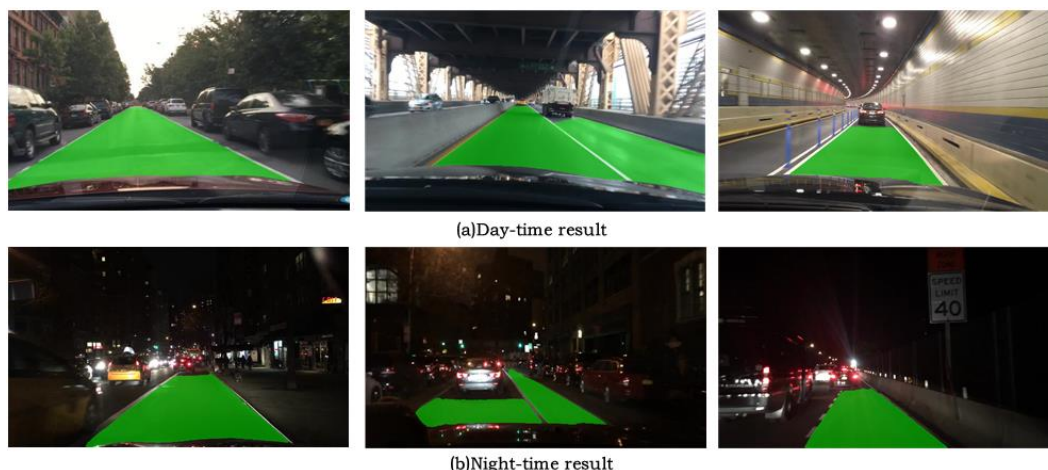
Fig 5. Drivable area segmentation results of DP-YOLO
