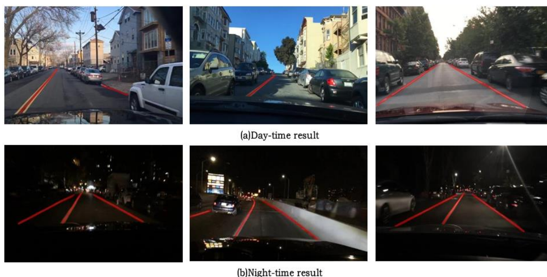
Fig 6. Lane line detection results of DP-YOLO
