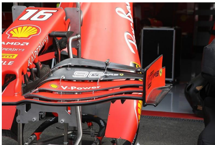
Figure 1. The front wing of a Ferrari F1 car with curved-line shape and flat surface [3]
