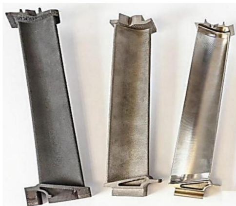
Figure 6. The 3D-printed TiAl blades for LPT of the GE90X engine.
