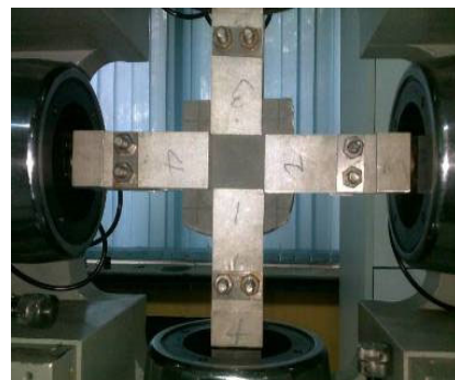
Figure 6. Bathtub type specimen test
