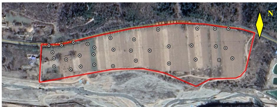
Figure 3. Layout of general detection points for soil layer thickness
