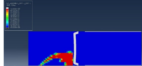
(b) Cleaning effect of the scraper when the interference fit is 2%
