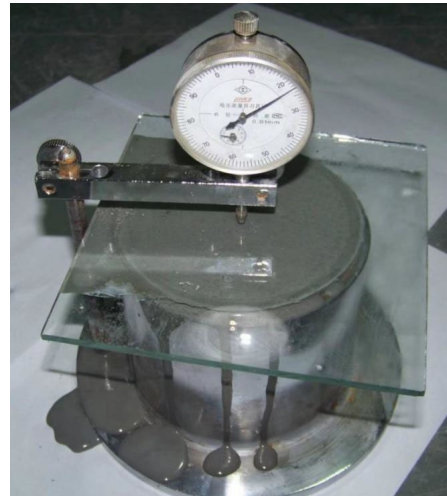
Figure 1. Vertical expansion ratio test
