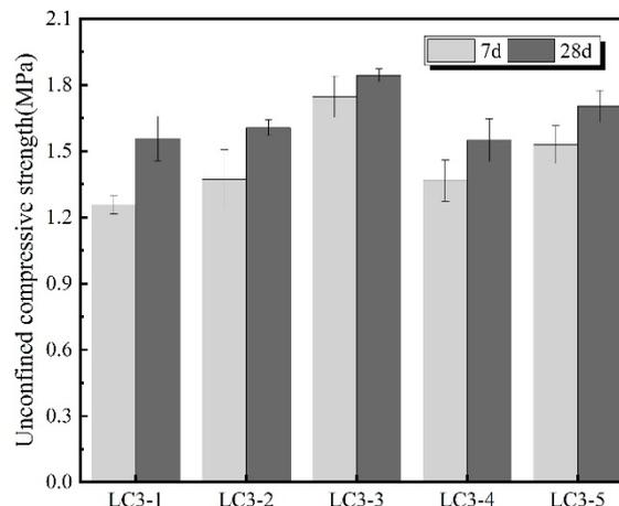
Figure 3. Effect of different components of LC3 solidified Zn contaminated soil on unconfined compressive strength
