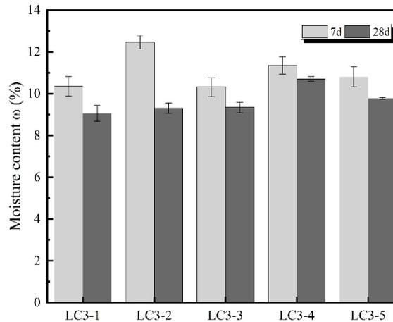
**Figure 1.** Effect of LC<sup>3</sup> solidification of Zn contaminated soil with different components on water content.
