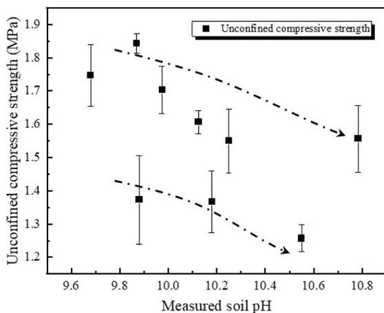
**Figure 5.** Fitting curve between unconfined compressive strength and measured soil pH of solidified Zn contaminated soil
