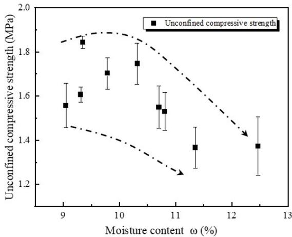
**Figure 4.** Fitting curve between unconfined compressive strength and moisture content of solidified Zn contaminated soil
