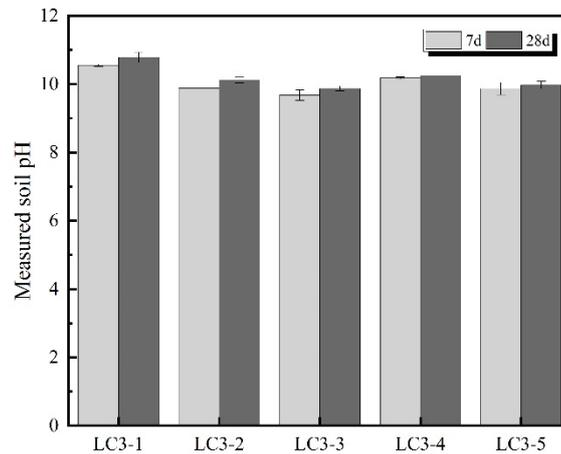
Figure 2. Effect of different components of LC3 on pH value of Zn contaminated soil
