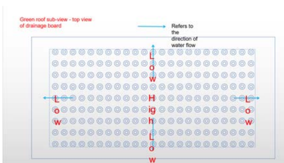
Figure 3. Green roof sub-view-top view of drainage board
